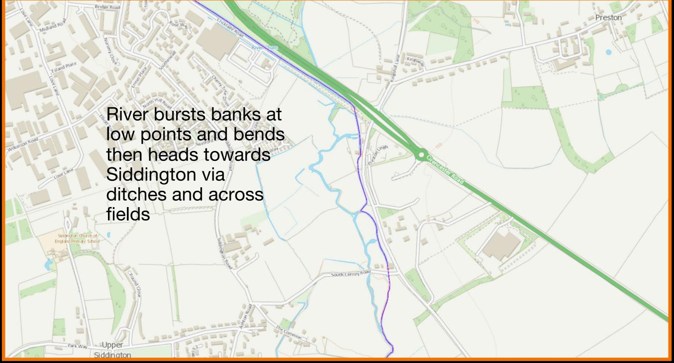
High rainfall over a prolonged time raises the river level and obstructions, blockages and limited capacity at Siddington Mill bridge forces the river to break its banks at low points
